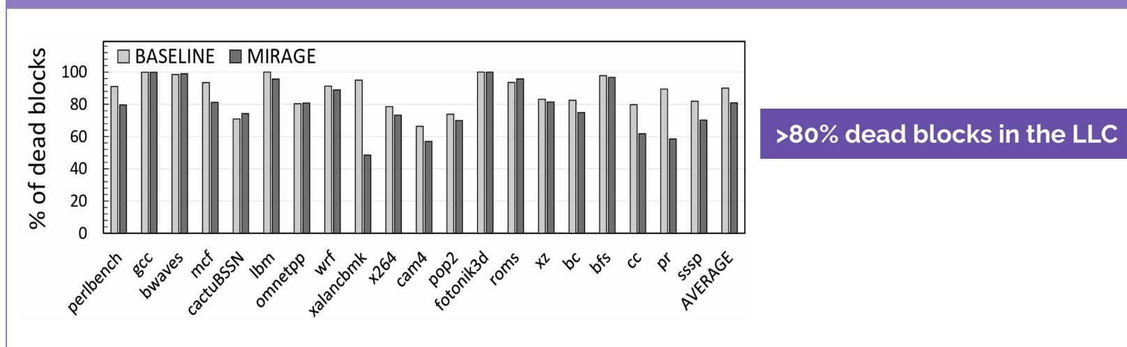
Naively reducing the data store size will lead to a large loss in performance  $\Rightarrow$  need a modification in the microarchitecture. Reuse Cache [2]: uses a larger tag store with two different types of tag entries: ones with only tag and the others with both tag and data.
