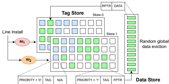
Fig. 2. Overview of the Maya cache design. White blocks represent invalid tag entries, yellow represents priority-0 tag entries, and green represents priority-1 tag entries.
