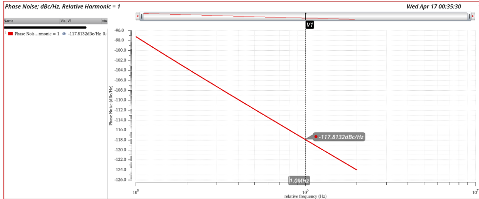
Figure 6: Phase Noise (in dBc) for the designed VCO circuit.
